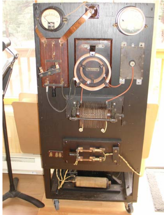
Spark gap transmitter made by K6GLH from period components
